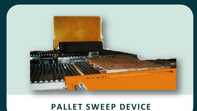
Systec's Pallet Sweep Device (PSD) is an efficient way to remove corrugated loads from pallets to infeed a machine. After the palleted load enters a zone, the pusher head is engaged and pushes the load off the pallet and onto the corresponding conveyor line. The load is then sent on for additional processing. After the head returns to the home position, the empty pallet is moved up the initial conveyor line to be cleared.
