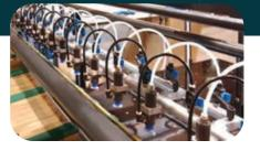
**TRAIL-EDGE LITHO FEEDER** Independent suction valves operate on one feed head providing fast set-up times and consistent feeding of lithosheets.
