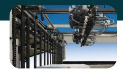
**TRAIL-EDGE LITHO FEEDER** Independent suction valves provide consistent feeding of litho-sheets, increased speed and fast set-ups.
