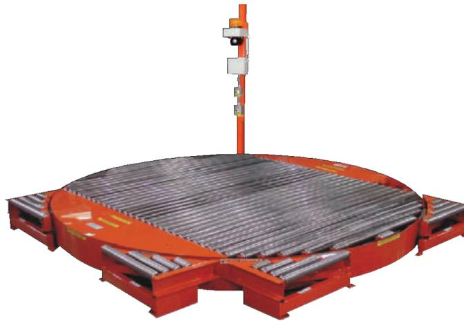
System's Center Pivot Conveyor (CPC) can be used at any point within the overall conveyor system. The CPC is primarily used where change in load direction is required, yet the load orientation must remain the same. This is particularly applicable where pallets may be used within the system. This is due to the fact pallets runners, or bottom boards, must remain perpendicular to the load carrying rollers to smoothly convey the load.
