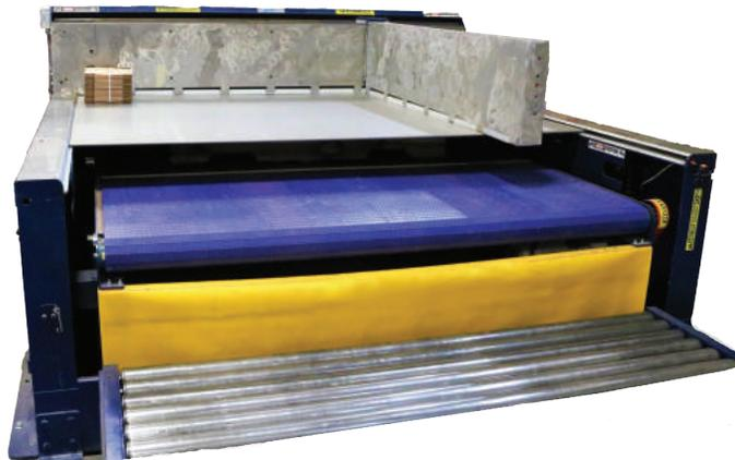
Systec's redesigned Load Former is an exceptional machine for ergonomic unit-load building. Operators can move bundles without lifting to build tiers to the finished unit-load.
