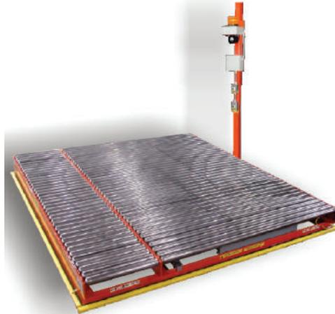
Systec's Side Pivot Conveyor (SPC) can be used at various points within the overall conveyor system. The SPC is primarily used where change in load direction is required, yet the load orientation must remain the same. This is particularly applicable where pallets may be used within the system. This is due to the fact that the pallet's runners, or bottom boards, must remain perpendicular to the load carrying rollers to smoothly convey the load.
