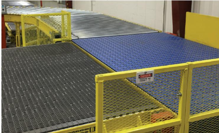
Systec's Performance Line Passive Right Angle Transfer or PLRAT is designed to allow for instantaneous transitions of loads, all while maintaining orientation. It is an alternative to belt transfers and allows for more flexibility and load building capabilities, all while maintaining a smaller foot print than a traditional 90° degree curve.
