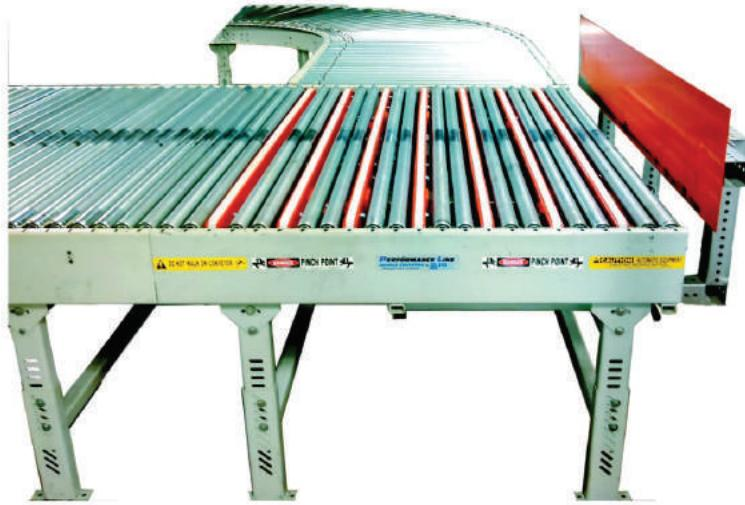
Systec's Performance Line Bundle Transfer / Ejector or the PBTE is unique in that it can integrate with vision inspection systems to allow for the quarantine of defective loads.
