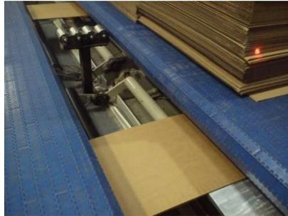
The system has a PLC program and sensors which measure the width of the load as it approaches the pad inserters. This information determines how the pads are positioned by the beam pad plates.
